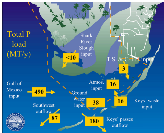
Figure 5.9 Estimates of the annual exchange of total phosphorus at Florida Bay's boundaries. Everglades estimates are annual median inputs to wetlands from canals (since 1979 for Shark Slough and since 1984 for Taylor Slough and the C-111 basin).
