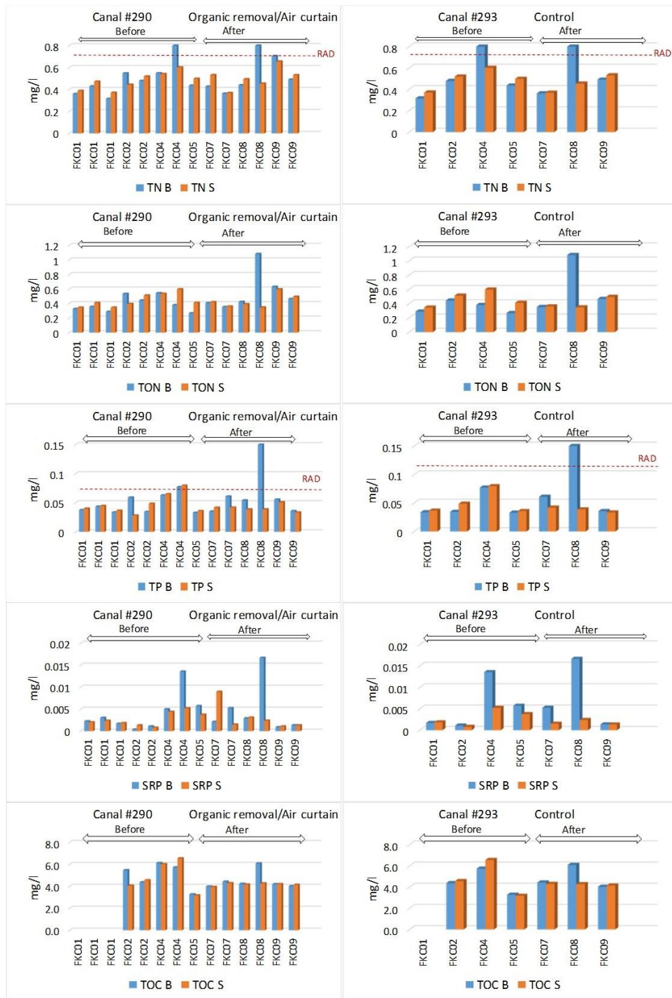
Fig 6.7.4. Water quality comparison between Before and After sampling, and between remediated Canal #290 and control Canal #293. Dissolved nitrogen species: total nitrogen (TN); total organic nitrogen (TON); total phosphorous (TP); soluble reactive phosphorous (SRP); and total organic carbon (TOC).
