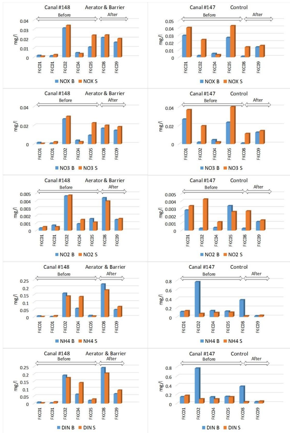
Fig 6.3.4. Water quality comparison between Before and AFTER sampling, and between remediated Canal #148 and control Canal #147. Dissolved nitrogen species: nitrate+nitrite (N+N), nitrate (NO 3 ), nitrite (NO 2 ), ammonium (NH 4 ) and dissolved inorganic nitrogen (DIN). Survey FKC09 occurred after Irma.
