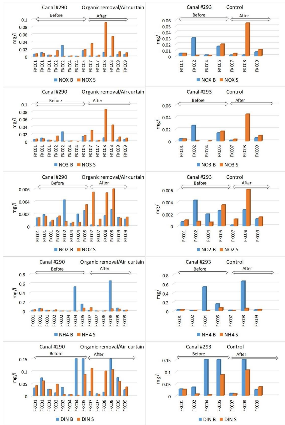
Fig 6.7.3. Water quality comparison between Before and After sampling, and between remediated Canal #290 and control Canal #293. Dissolved nitrogen species: nitrate+nitrite (N+N), nitrate (NO 3 ), nitrite (NO 2 ), ammonium (NH 4 ) and dissolved inorganic nitrogen (DIN)
