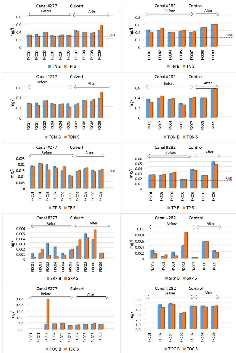
Fig 6.5.4. Water quality comparison between Before and After sampling, and between remediated Canal #277 and control Canal #282. Dissolved nitrogen species: total nitrogen (TN); total organic nitrogen (TON); total phosphorous (TP); soluble reactive phosphorous (SRP); and total organic carbon (TOC). Survey FKC09 occurred after Irma
