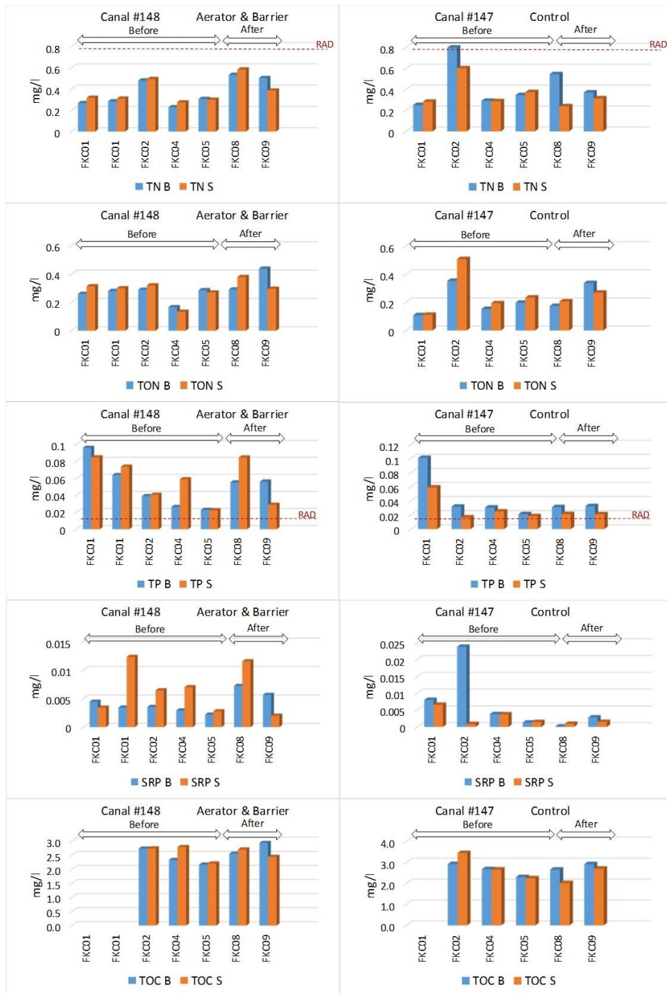
Fig 6.3.5. Water quality comparison between Before and AFTER sampling, and between remediated Canal #148 and control Canal #147. Dissolved nitrogen species: total nitrogen (TN); total organic nitrogen (TON); total phosphorous (TP); soluble reactive phosphorous (SRP); and total organic carbon (TOC). Survey FK09 occurred after Irma
