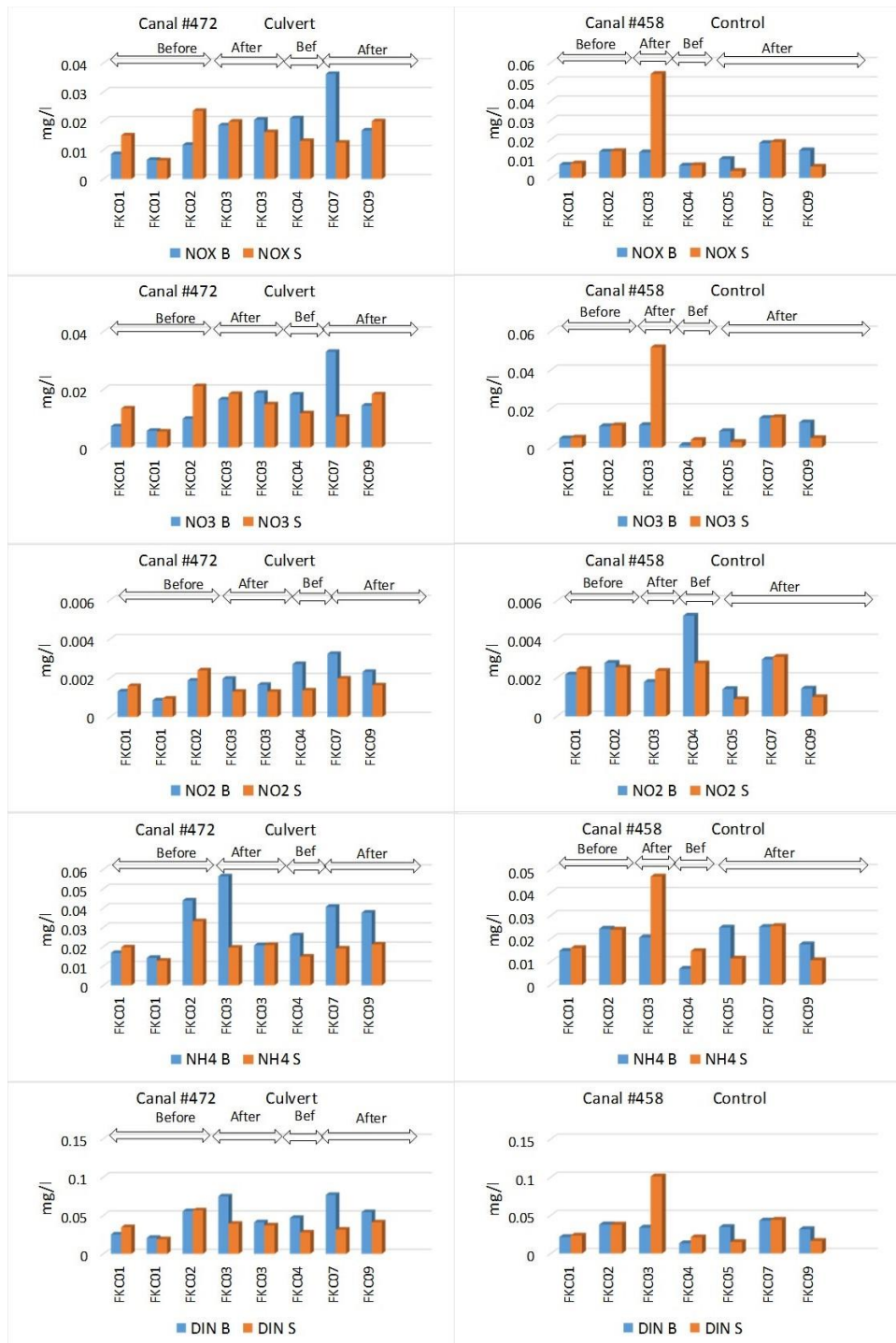
Fig 6.8.4. Water quality comparison between Before and After sampling, and between remediated Canal #472 and control Canal #458. Dissolved nitrogen species: nitrate+nitrite (N+N), nitrate (NO 3 ), nitrite (NO 2 ), ammonium (NH 4 ) and dissolved inorganic nitrogen (DIN)
