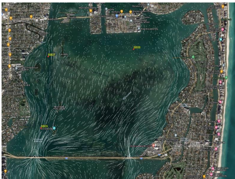
Figure 73 Velocity field in the area limited by the 195 highway to the south and SR 934 to the north. Note the higher velocities through the 195 bridges and the circulation patterns with large eddies.
