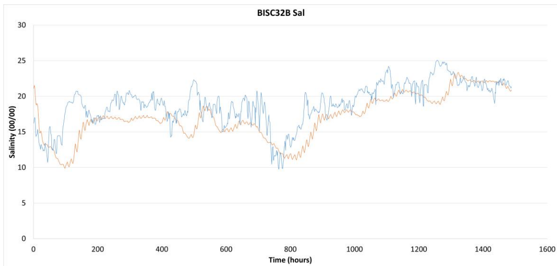
Figure 111 Comparison of salinities at station BISC32B. Blue lines are model results, Orange line are observations.
