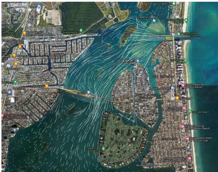
Figure 72 Velocity field near the northern end of Biscayne Bay. Haulover is the northern open boundary in the model.
