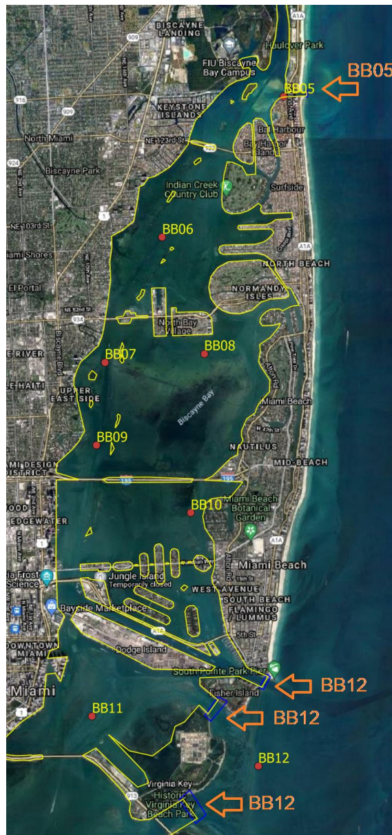
Figure 42 Boundary Condition Data Used in the Northern part of Biscayne Bay Model.
