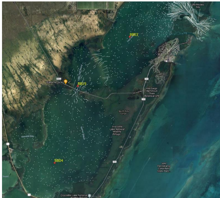
Figure 78 Velocity field on the southern part of the model. This area includes Card Sound and Barnes Sound. Rhodes Key is the southernmost open boundary in the model.
